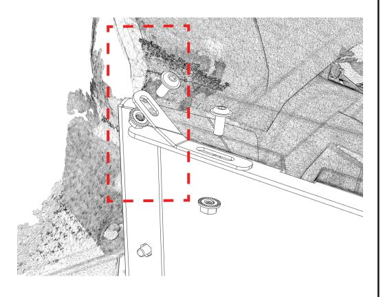
You have now completed the installation of the first floorboard. - Don't forget to retighten all screws!
