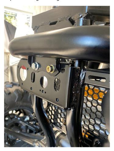
Install the long 80 mm spacer and use blue Loctite on the threads.
