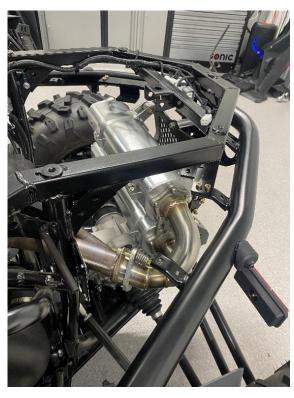
Use the supplied M8 X 70 bolts and washers and re-use the OEM springs to connect the header and RJWC pipe.
