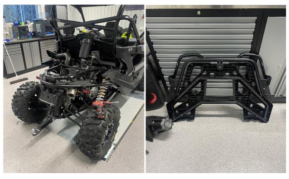
Remove the factory muffler, see the pictures below on where the brackets/hangers are located and where the header connects to the muffler there is a spring loaded coupling where you need to remove the bolts. On the new exhaust you re-use the springs but with longer bolts we supply.
