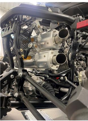
We recommend installing the muffler package after you have installed the bracket.
