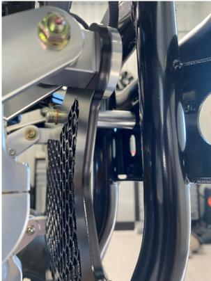
Install the BRKT-044 bracket. See the picture below. NOTE you have to install the rear plastics back together with the RJWC muffler bracket if you want to use the plastics. Use M6 Washers between the vehicle and the BRKT-044 if you don't use the factory plastics to cover up the gap so that you can tighten it down without bending the brackets.
