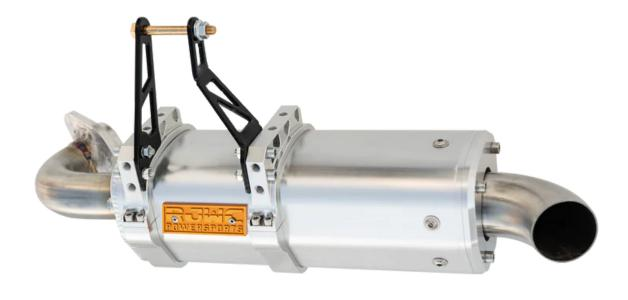
Step 5 - Use the above image to ensure the pipe is correctly mounted to the APX can.
