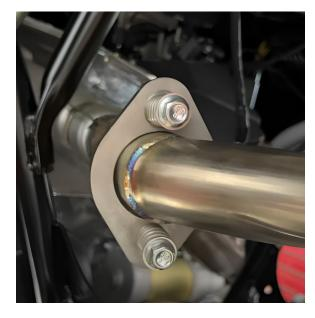
Step 7 Use the two exhaust bolts that were removed with the stock exhaust to secure the exhaust pipe flange in place.
