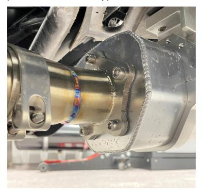
Step 4 – Install the mid pipe on the header pipe, use the supplied graphite gasket and the exhaust springs. We recommend that you use an exhaust spring tool.
