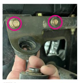
**STEP 3.** With the stock exhaust removed, you can now remove the stock exhaust bracket.
