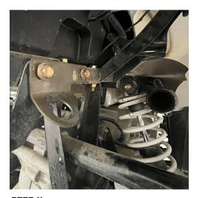
Install the Black Exhaust Bracket into the same location as the stock bracket using the stock bolts.
