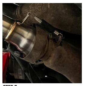
Use the 2x RJWC Exhaust Springs to connect the pipes, and replace the stock pins that were removed with the stock exhaust with the replacement Aluminium pins.
