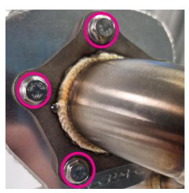
**STEP 3.**Place the Exhaust Gasket between the pipe and the APX can and use 5x M6 Flange Screws to secure the pipe to the APX can.
