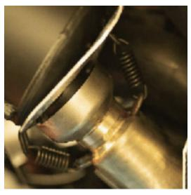
**STEP 1.** To remove the stock muffler, start by removing the two springs.
